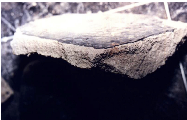
Figure 15. Extracted mortar layer fragment of a ceramic tiling.
