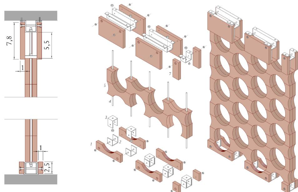
This refers to a pre-fabricated construction system based on porcelain stoneware pieces that uses steel turnbuckles to join one to the other so they can be rolled up for transportation before being fitted. They are of great use in rehabilitation projects for translucent and permeable partitions given their light weight and clean aesthetics.
