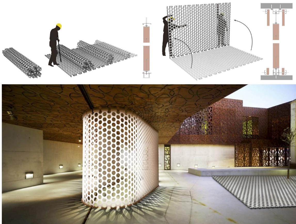
The result is a dry-fitted lattice with many applications and especially attractive for designing interior partitions, which, furthermore, can be varied in configuration and size over time by simply fitting new parts or removing those that are no longer needed.
