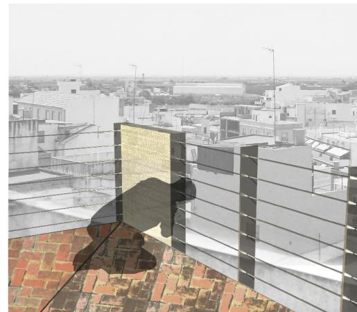
This is an original solution for the breastwork on old buildings. Given that it is dry-fitted with non-aggressive fastening to the support structure, it provides excellent performance in earthquakes to prevent such traumatic experiences as in the town of Lorca (Spain) in May 2011. It would use the obsolete stock of ceramic pieces that are no longer marketable.
