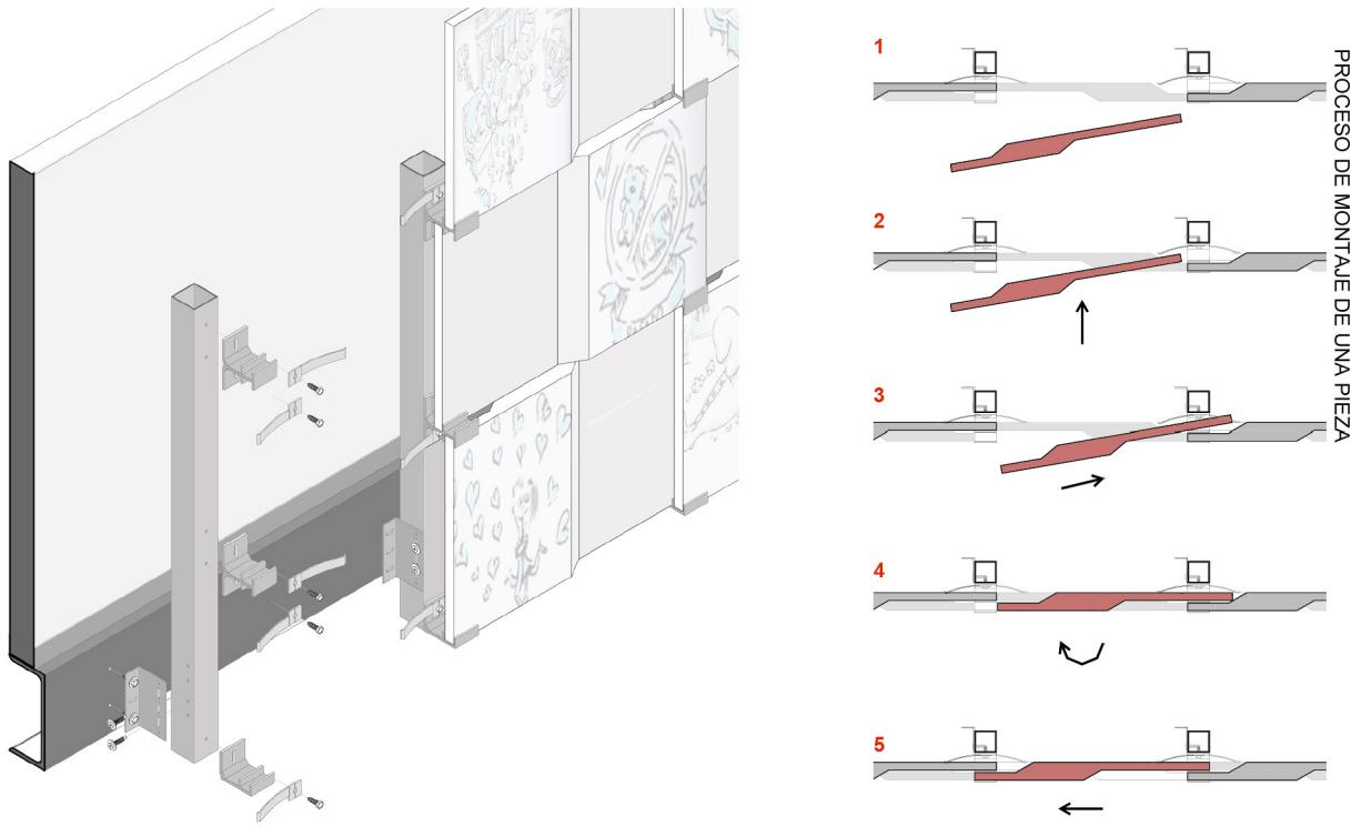
At the same time, a tile anchoring system has been designed so that tiles can be (re)moved one by one. The system thus developed allows for tiles to be removed and subsequently refitted or reused on other cabins or buildings.
