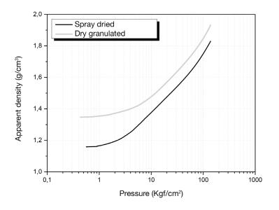
Figure 1. Compaction behaviour of spray-dried and dry-granulated powders.
