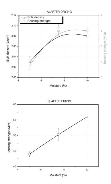
Figure 2. Effects of the moisture content in the dry granulated powder on the mechanical behaviour of the bodies.
