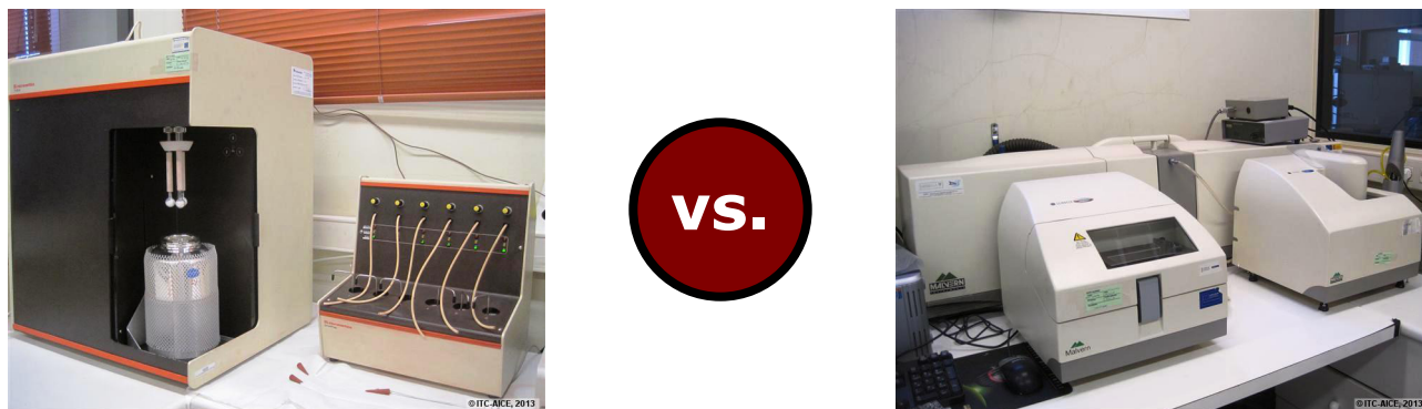
Figure 3. instruments for the determination of the specific surface area of materials a) Nitrogen adsorption instrument, b) Wet laser diffraction instrument.
