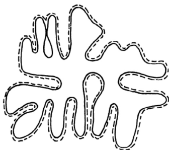
Figure 1 Specific surface area of an irregular particle.
