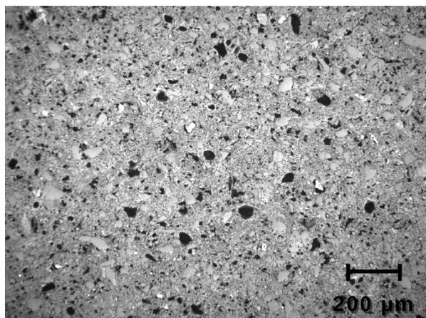
Figure 3. Microstructure of the fired piece formed with spray-dried powder GR.
