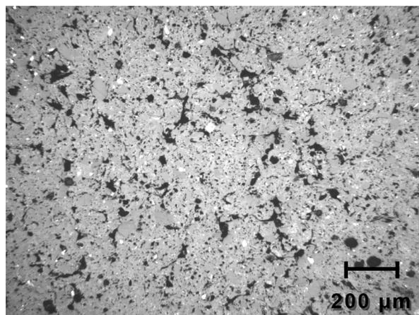
Figure 4. Microstructure of the fired piece formed with granulate GR.
