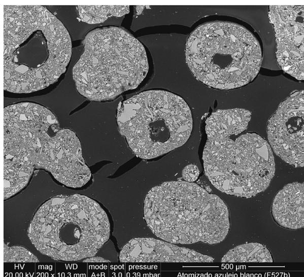
Figure 1. Microstructure of spray-dried powder AB.
