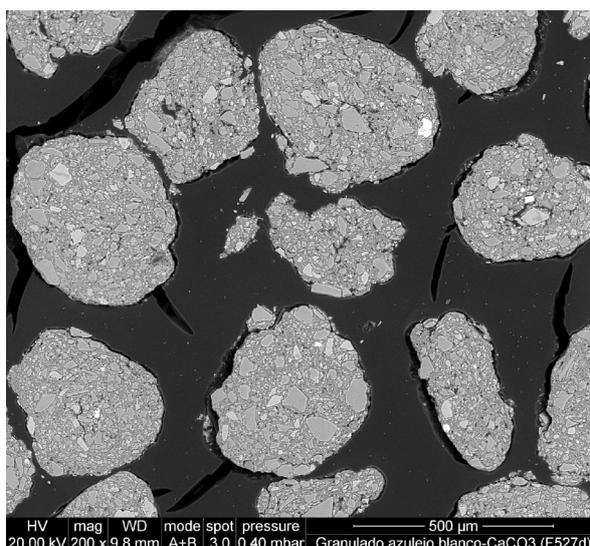
Figure 2. Microstructure of granulate AB.
