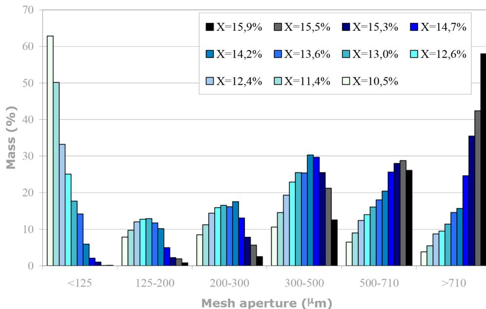
Figure 3. Evolution of the particle size fractions on modifying the granulation water addition.
