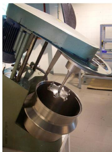
Figure 1. Image of granulator with rotor pin1.
