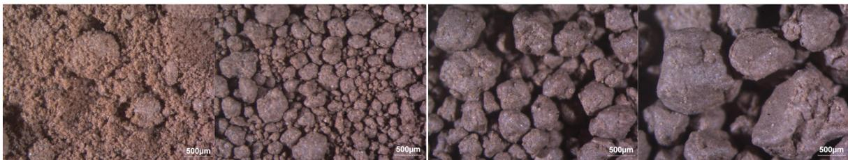
Figure 2. Pictures of granules obtained at different moisture contents (% on a dry basis).
