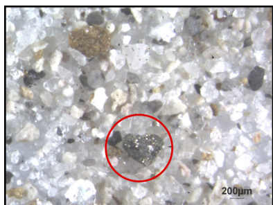
Figure 4. Magnifying glass photograph of pyrite traces in the clay sample.
