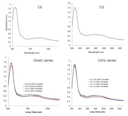
Figure 4. Diffuse reflectance spectra of the monoporosa glazings.
