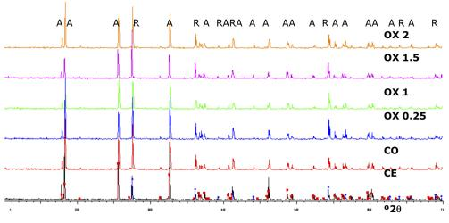
Figure 1. X-ray diffraction (A=Armalcolite (MgFe)(FeTi<sub>3</sub>)O<sub>10</sub>, R=Rutile TiO<sub>2</sub>).
