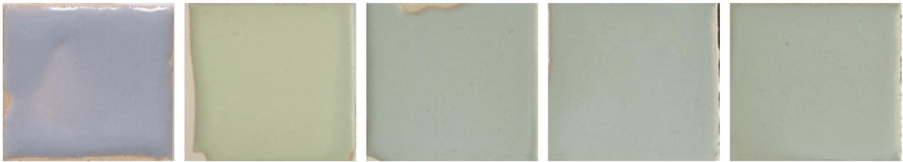
CE Double firing 66/-0,5/-2,3      CE Monoporosa 71.5/-0.2/13.9      CO Monoporosa 67.1/-0.7/4.8      CIT 0,25 Monoporosa 69.3/-1.0/4.4      OX 1,5 Monoporosa 66.5/-0.2/6.0
