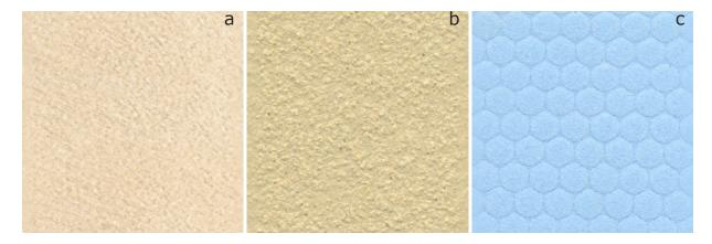
Figure 15. Tested ceramic tiles: a) smooth with roughness, b) textured, c) embossed.
