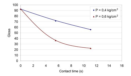
Figure 5. Surface gloss as a function of contact time at different pressures.
