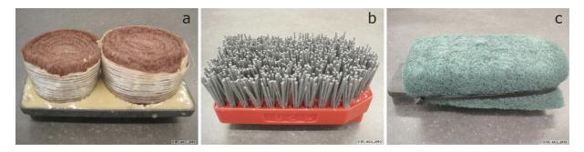
Figure 3. Abrasive materials used: a) sanding brush, b) SiC brush, c) commercial scouring pad.
