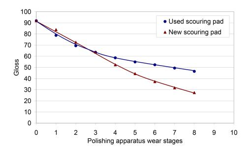
Figure 7. Surface gloss as a function of the wear stage either reusing the scouring pad or changing it after each wear stage.
