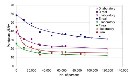
Figure 13. Correlation of the polishing apparatus wear method with the in situ study in the indoor building area with direct outdoor access.
