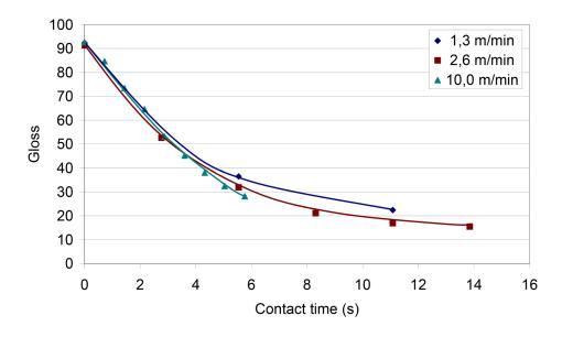
Figure 6. Surface gloss as a function of contact time at different belt rates of advance.
