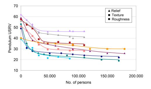
Figure 14. Life span of the slip-resistance performance of different types of ceramic tiles.
