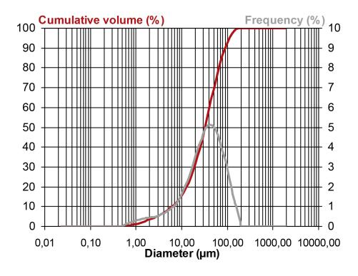
Figure 4. Particle size curve of the powder obtained on calcining the commercial scouring pad.
