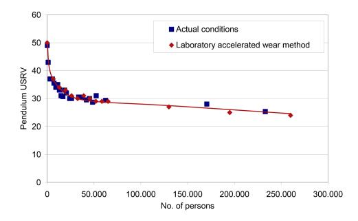
Figure 10. Correlation of the polishing apparatus wear method with actual conditions for the outdoor flooring.
