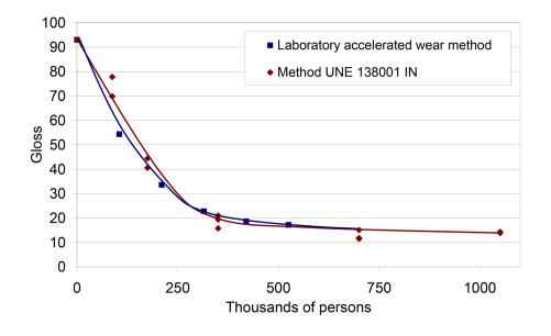
Figure 8. Correlation of the accelerated wear method with method UNE 138001 IN.
