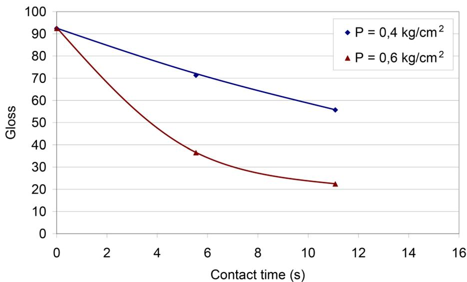
Figure 5. Surface gloss as a function of contact time at different pressures.
