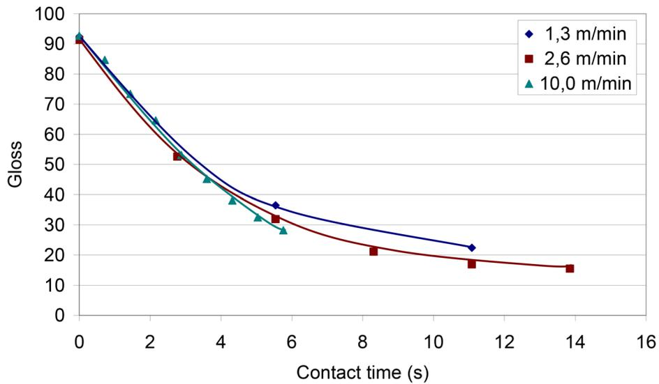
Figure 6. Surface gloss as a function of contact time at different belt rates of advance.
