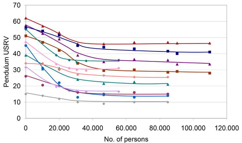
Figure 12. Evolution of slip resistance of the flooring installed in the university cafeteria.
