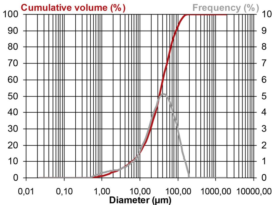
Figure 4. Particle size curve of the powder obtained on calcining the commercial scouring pad.
