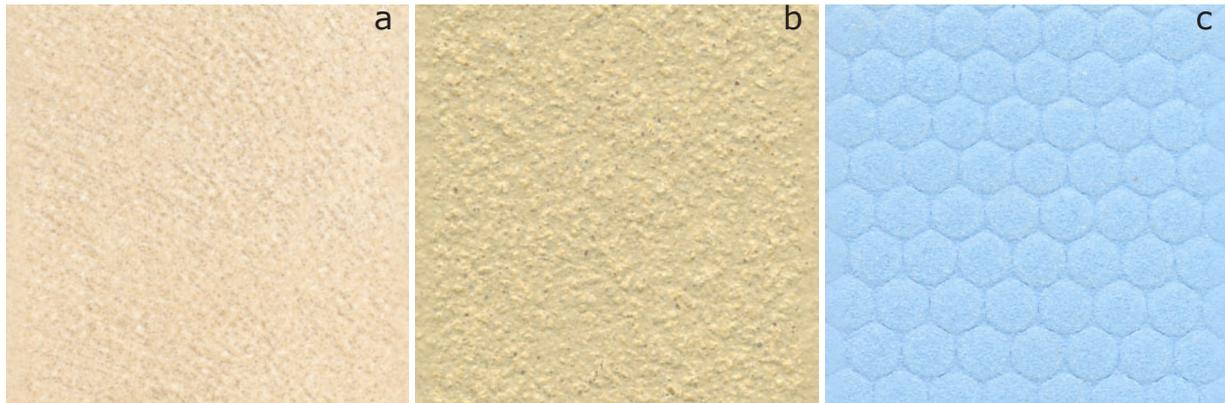
Figure 15. Tested ceramic tiles: a) smooth with roughness, b) textured, c) embossed.
