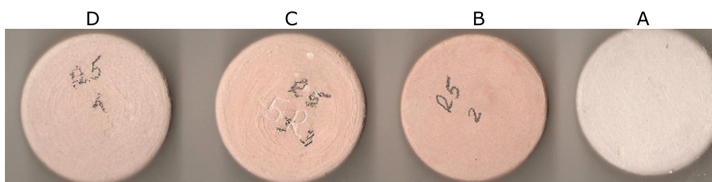
Figure 1: Pictures of the samples before and after the sintering stage: A – Sample before sintering; B – Sample sintered at 900°C; C – Sample sintered at 1000°C; D – Sample sintered at 1100°C.
