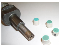
Figure 2. Samples and 6 mm drill bit for obtaining ceramic surface samples
