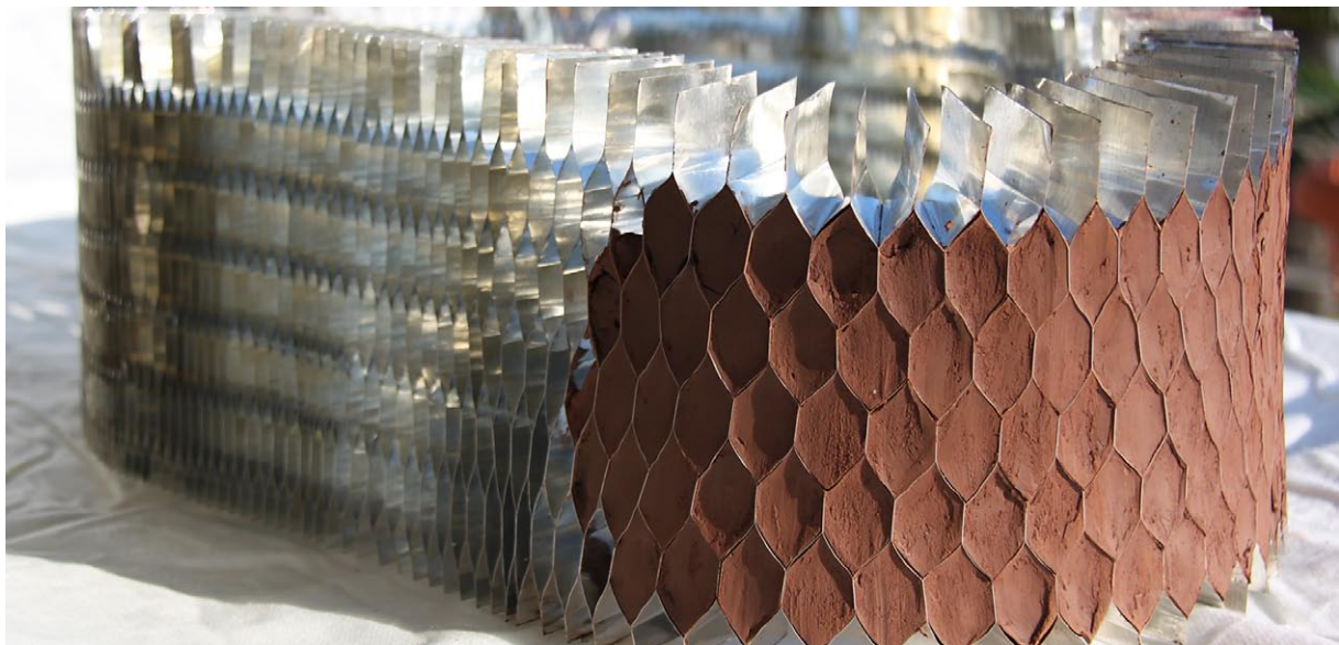
Fig. 1.25 | System test material. NEX mesh + Ceramic pieces
