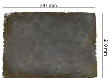
Fig. 3.03 | The sequence of flat panel composite (Honeycomb + Fine Art Cement)
