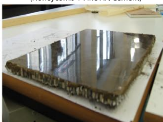
Fig. 3.04 | The sequence of flat panel composite (Honeycomb + Glass Fibre Sheet + Fine Art Cement)
