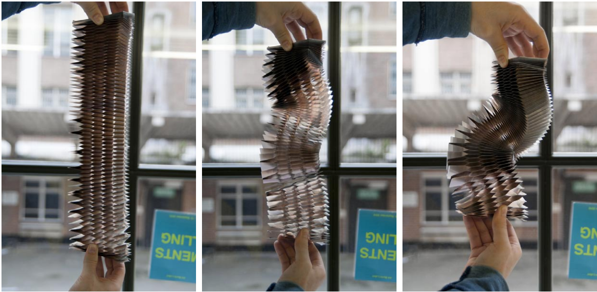
Fig. 1.19 | Sample of NEX Aluminium Honeycomb Panel.
