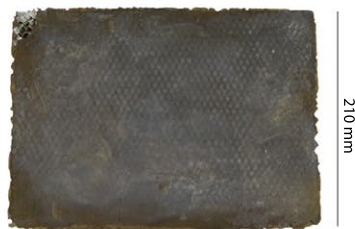
Fig. 3.03 | The sequence of flat panel composite (Honeycomb + Fine Art Cement)
