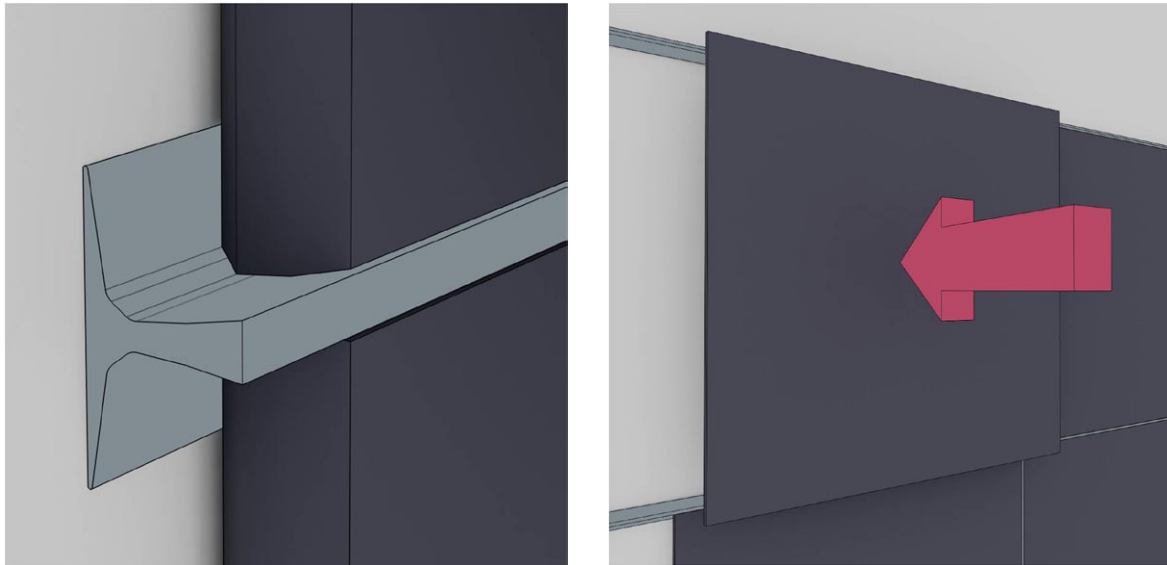
Figure 10. Scheme of the rigid joint system assembly
