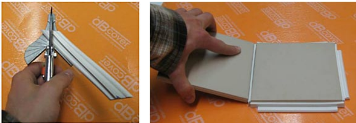
Figure 4. Prototypes of the joint and groove system
