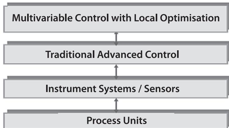
That means that the process is controlled by means of traditional loops, basically PID controllers, which operate at second intervals. Some items in cascade and with modified feed-forward operate at slightly longer time intervals and form part of the Traditional Advanced Control. Then comes Multivariable Control, which combines data from sensors and analysers to establish local optimisation settings. These controls operate at minute intervals.
