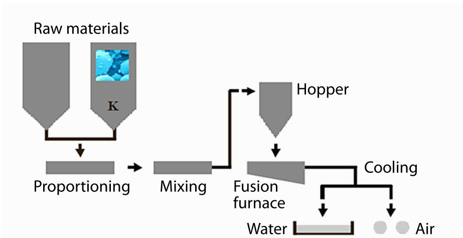
The process starts when previously selected and measured raw materials are fed in pre-determined proportions. They are transferred on a pneumatic conveyor to a mixer and from there are fed into the melting furnace, where the actual fritting process takes place.
