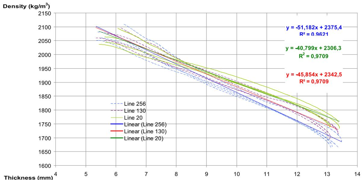
Illustration 8. Da vs. thickness for flat back (only up-flanks)
