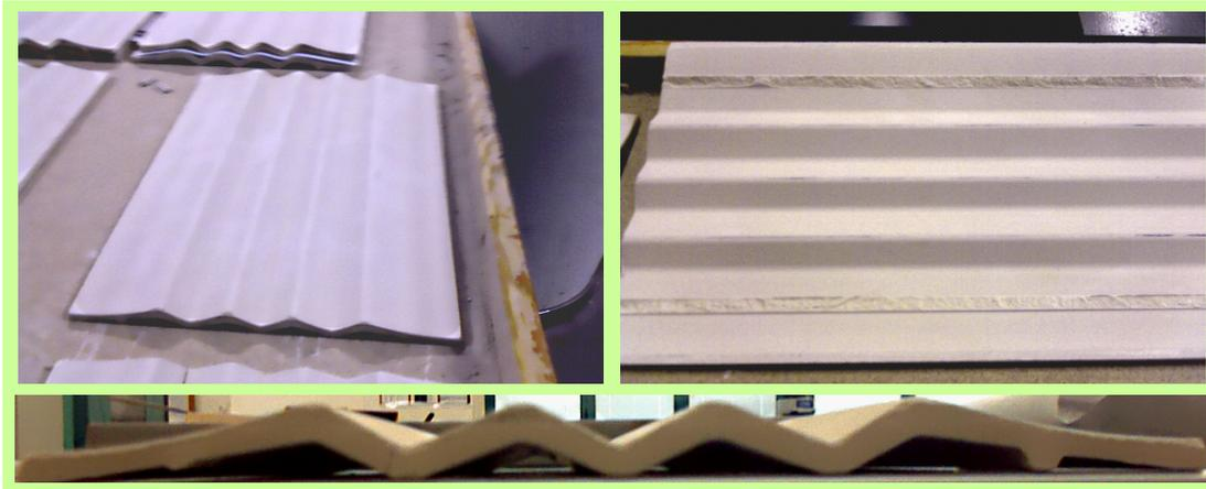
Illustration 3. Pressed prototypes of the piece with compensated back (reservoir)
