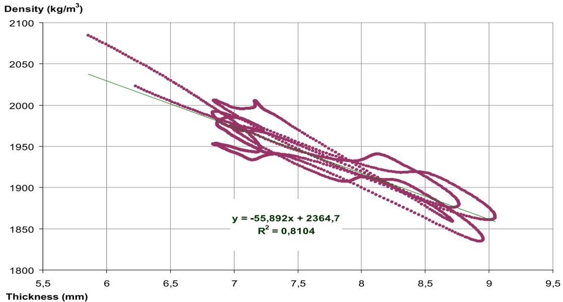
Illustration 7. Da vs. thickness for shaped back (reservoir) (all points) line 17
