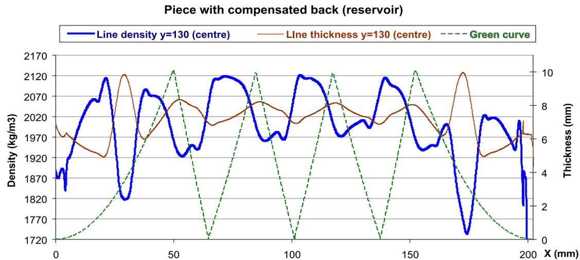
Illustration 6.  $D_a$  and thickness in a piece with compensated back (reservoir)
