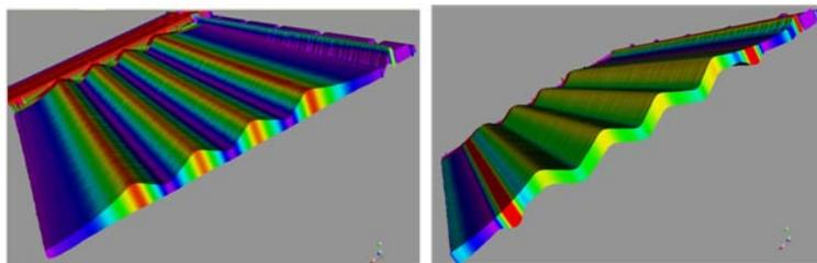
Illustration 4. Measurement of green thickness. Flat back and with reservoir
