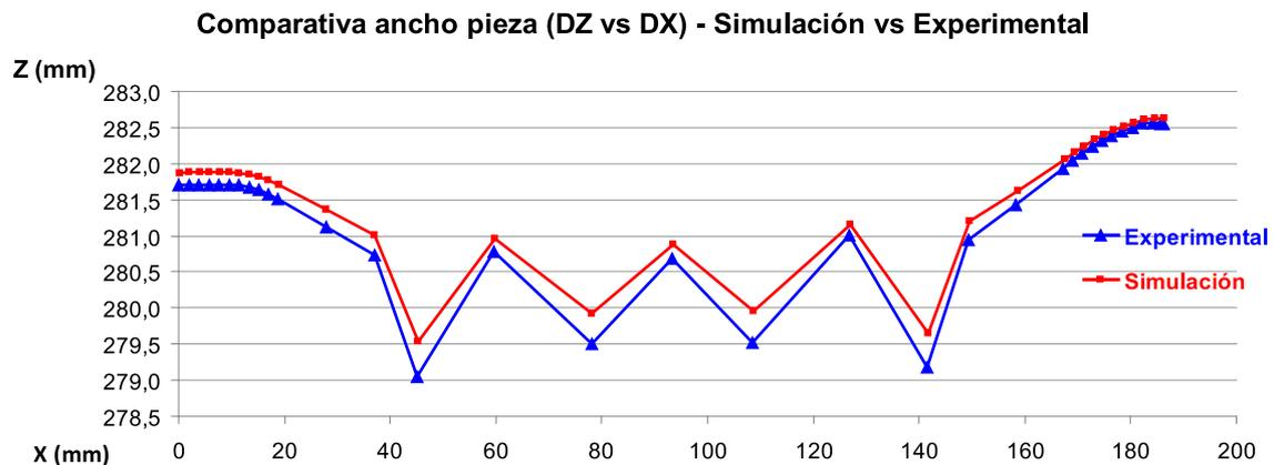
Illustration 10. Final dimensions of the pieces in width ( $L_i$  values in Illustration 9) real/simulation
