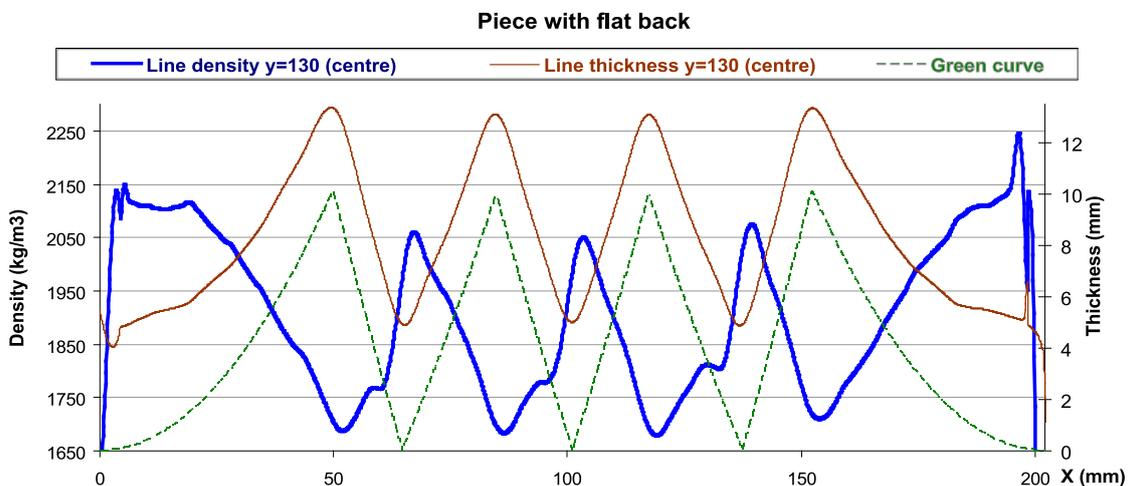
Illustration 5.  $D_a$  and thickness in a piece with flat back
