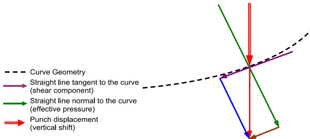
Illustration 1. Components of the pressing force in curved surfaces.
