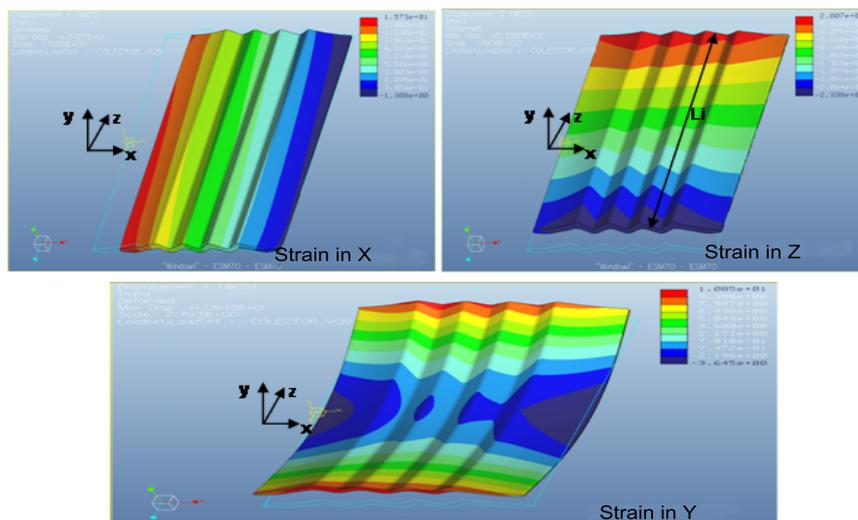
Illustration 9. Values of the strains in each axis with strain in simulated pieces.
