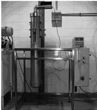
Figure 4 Assembly for the measurement of the dustiness of bulk materials by the continuous fall method. Schematic illustration of the test assembly parts.
