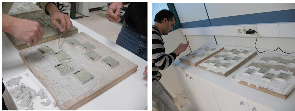
Figures 2,3. Fixing of the test pieces on the substrate.
