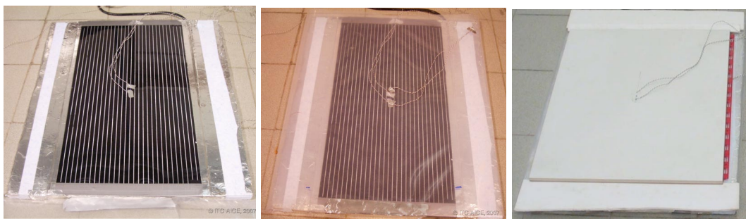
Figure 3. Photos showing the installation of the measuring thermocouples on the heating element (left), the polyethylene substrate (centre), and the tile (right).
