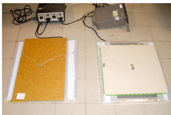
Figure 5. General photo of the assembly showing the difference in dimensions between the cork tile and the CT system.
