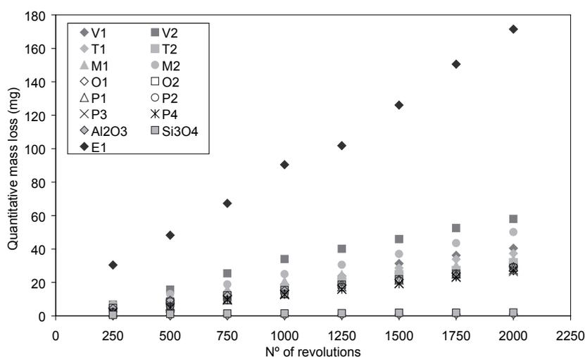
Figure 2. Representative graph of the wear resistance of the tested materials.
