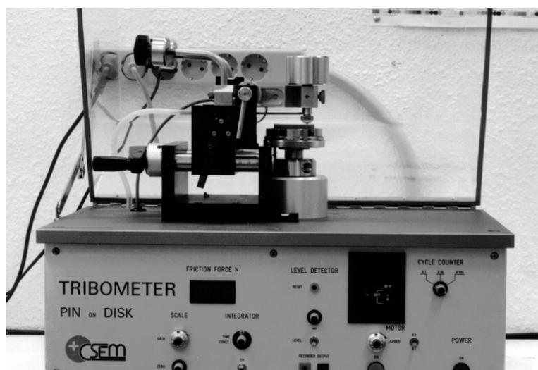
Figure 1. Pin-on-disk tribometer.
