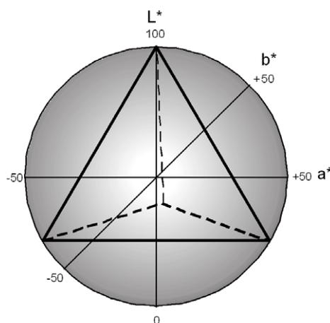
Figure 8. Schematic illustration of the largest tetrahedron that could be fitted into the simplification of the CIELab space.
