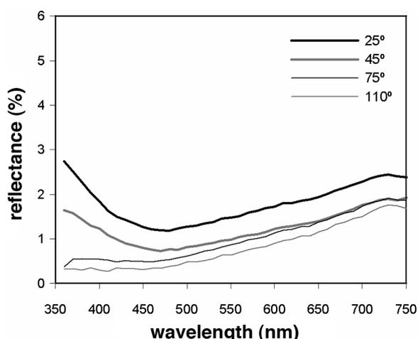
Figure 3. Evolution of reflectance versus wavelength and measurement angle for glaze A19.
