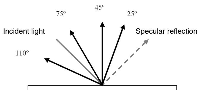
Figure 1. Schematic illustration of the incident angles (45° in relation to the normal) and measurement angles (25°, 45°, 75°, and 110° in relation to the specular reflection) of the goniospectrophotometer used.
