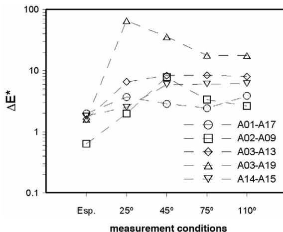
Figure 7. Colour differences  $\Delta E^*$  for different pairs of glazes as a function of the instrument used.
