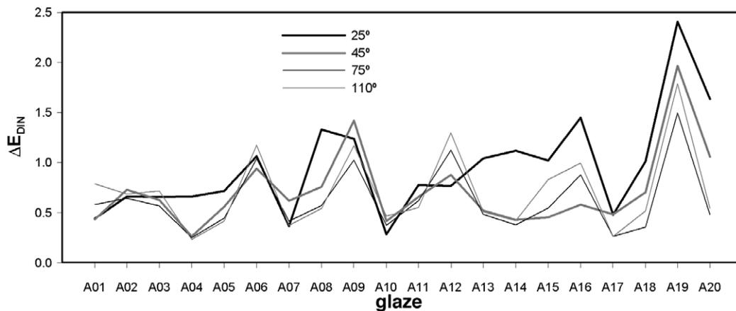
Figure 4. Colour difference  $\Delta E_{DIN}$  between the different measurements with respect to the average in each 'metallised' glaze (according to standard DIN 6175-2).
