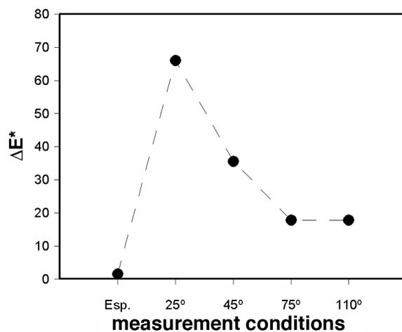
Figure 5. Colour differences  $\Delta E^*$  between glazes A03 and A09 as a function of the instrument used (Esp. is the spectrophotometer; the angles correspond to the goniospectrophotometer).
