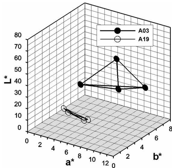
Figure 6. Situation in the CIELab space of the chromatic coordinates of glazes A03 and A19, evaluated at the four angles of the goniospectrophotometer.
