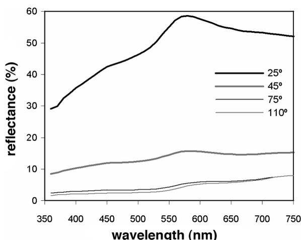
Figure 2. Evolution of reflectance versus wavelength and measurement angle for glaze A03.
