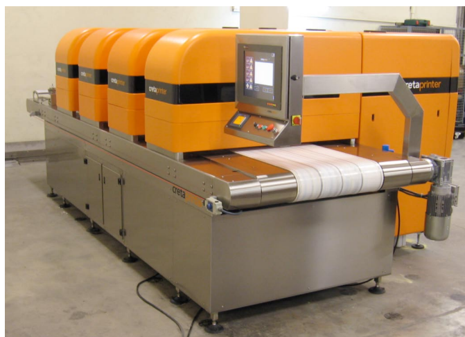
Figure 9. Example of a commercial in-line single-pass printer (Cretaprinter: image from Xaar plc).
