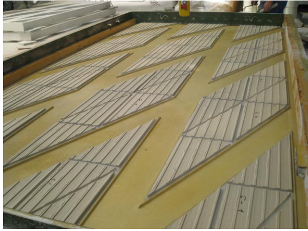
Figure 8. Installation of ceramics in the mould.
