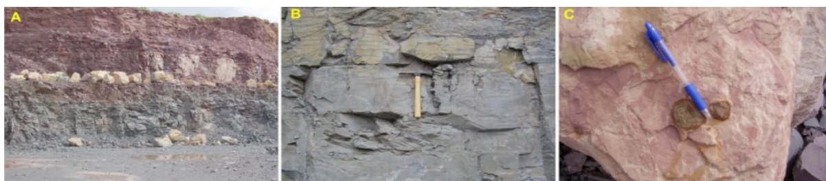
Figure 1. (A) General view of the mine where the sample was collected. (b) Detail of the material rich in organic matter. (c) Altered pyrite nodule found next to sandstones, where there are also fractures occupied by calcite.
