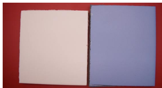
Figure 4. Tiles before (left) and after (right) application of a soluble colour.
