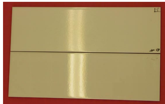
Figure 3. Tiles before (below) and after (above) application of nanometric aluminium oxide.
