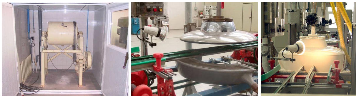
Figure 6. View of the mill used for the trials, and bell waterfall used in the trials before and during the glazing process.
