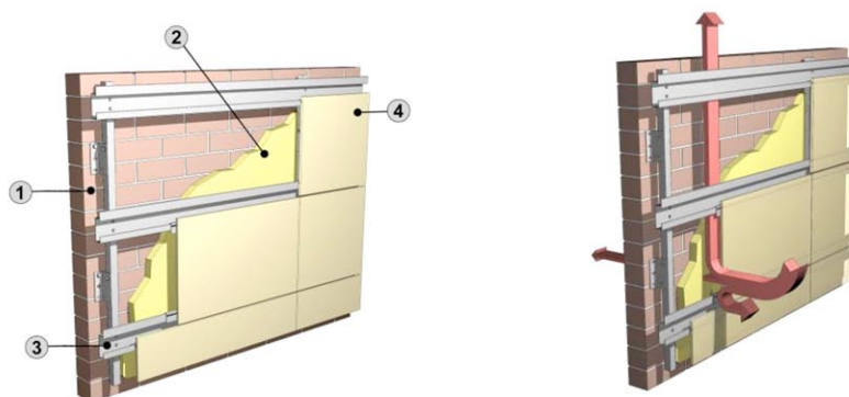
a) Construction detail.
