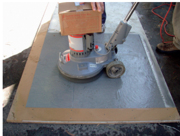
(a) Polishing/buffing machine used to wear tiles
