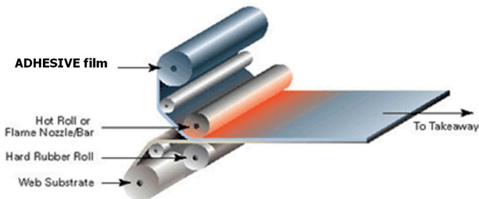
Figure 7. Hot Roll/Belt Lamination
