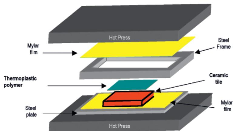
Figure 1. Scheme of laboratory ceramic tile heat lamination
