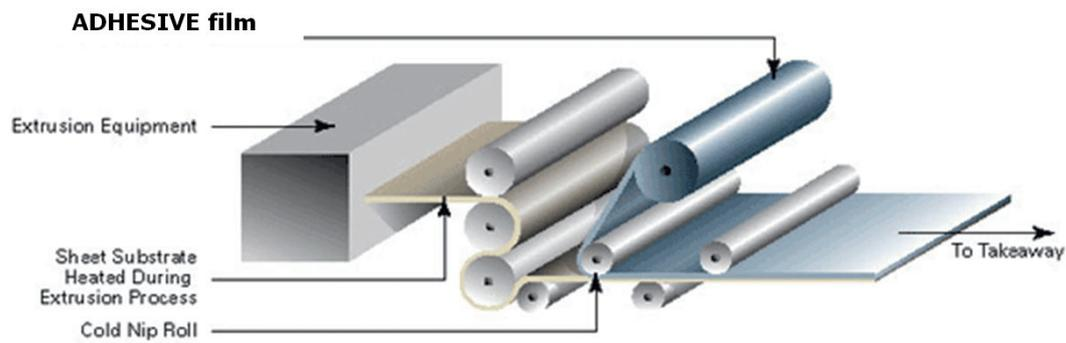
Figure 8: Sheet (or tiles) Extrusion.
