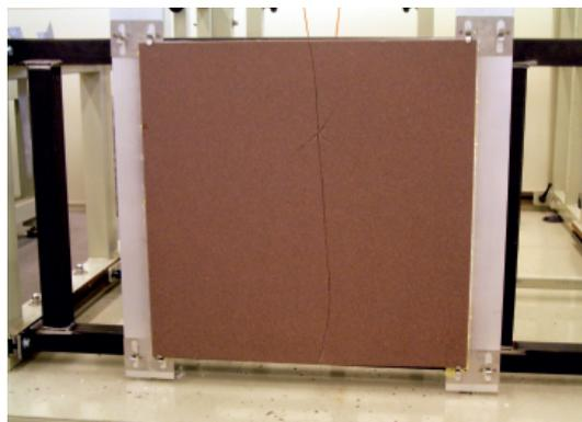
*Figure 5. Film laminated Tile broken at 10 Joule*
