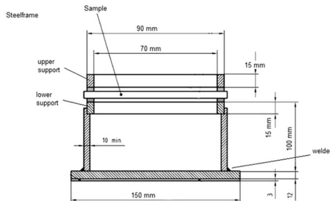
Figure 2. Supporting frame for ball drop test
