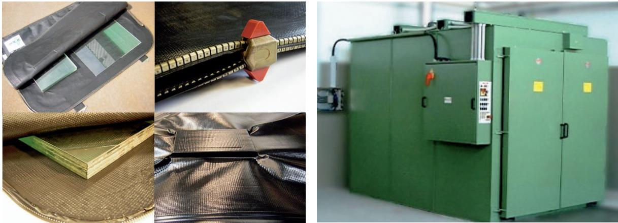
Figure 9. Vacuum lamination for glass sandwiches. Left: vacuum bags. Right: oven <sup>[6]</sup>.
