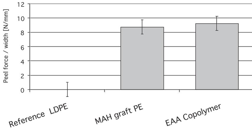
Chart 1. Adhesion of functional polymer film to ceramic tile in 180° peel test
