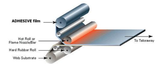
Figure 7. Hot Roll/Belt Lamination
