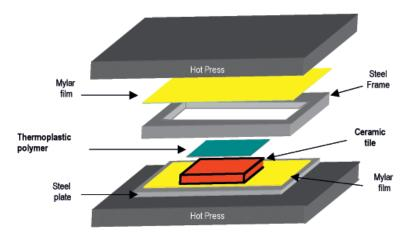
Figure 1. Scheme of laboratory ceramic tile heat lamination
