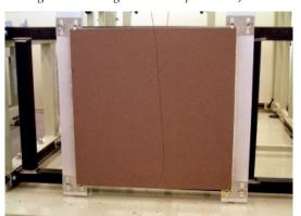
Figure 5. Film laminated Tile broken at 10 Joule
