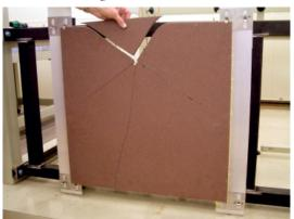
Figure 4. Breakage with loose piece at 3 Joules
