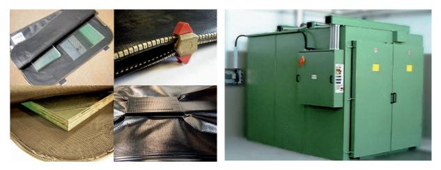
Figure 9. Vacuum lamination for glass sandwiches. Left: vacuum bags. Right: oven <sup>[6]</sup>.
