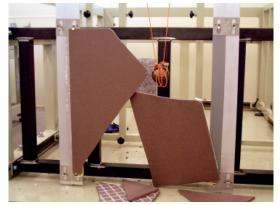
Figure 6. Ceramic tile broken at 10 Joule
