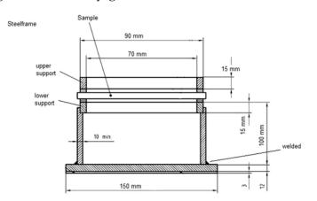
Figure 2. Supporting frame for ball drop test
