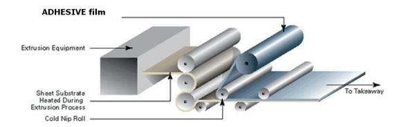
Figure 8: Sheet (or tiles) Extrusion.
