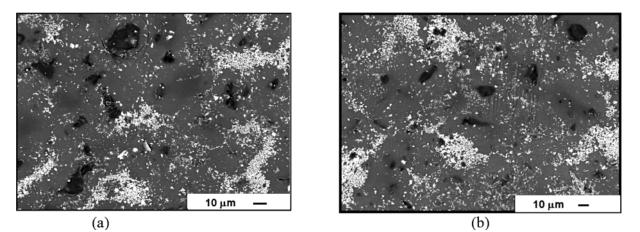
*Figure 2. Representative BE images of the standard formulation (M) and wt. % pegmatite containing formulation (M-20). (a) M and (b) M-20*
