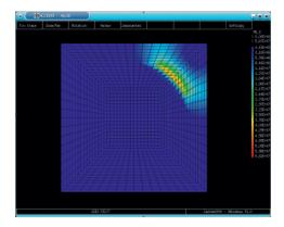
Figure 1. Main deformation and strain under load concentrated in the corner.
