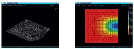
Figure 2. Main deformation and strain under load concentrated on the centre of the edge.
