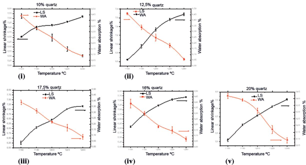
Figure 3. Vitrification curve (i) M1, (ii) M2, M3 (iii), M4 (iv), M5 (v).
