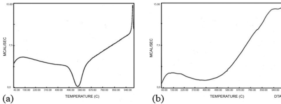
Figure 2. Differential thermal curves (DTA) of the powder: (a) kaolin, (b) sodium feldspar.
