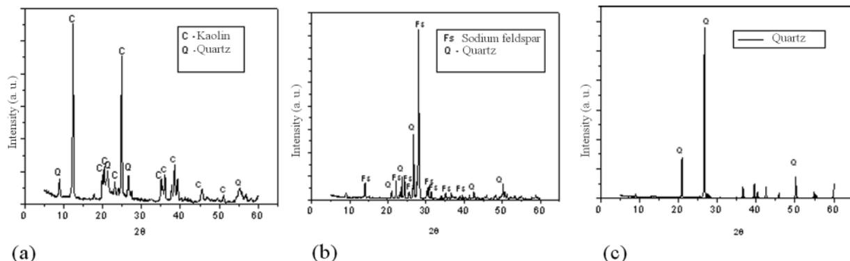
Figure 1. X-ray diffractograms of the raw materials: (a) kaolin, (b) sodium feldspar (c) quartz.
