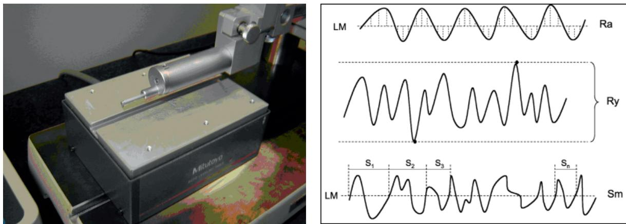
Figure 1. Mechanical contact profilometer and roughness indicator parameters that can be obtained from the measured profiles
