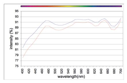
Figure 2. Reflectance for the white glaze before (blue line) and after (red line) abrasion (12000 cycles)
