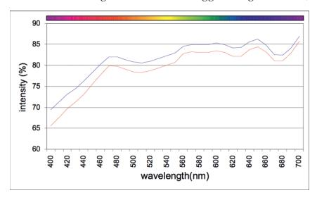
Figure 4. Reflectance for the transparent glaze before (blue line) and after (red line) abrasion (12000 cycles)
