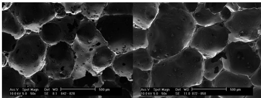
Figure 2. Microstructure after sintering for 850°C and 900°C firing temperatures
