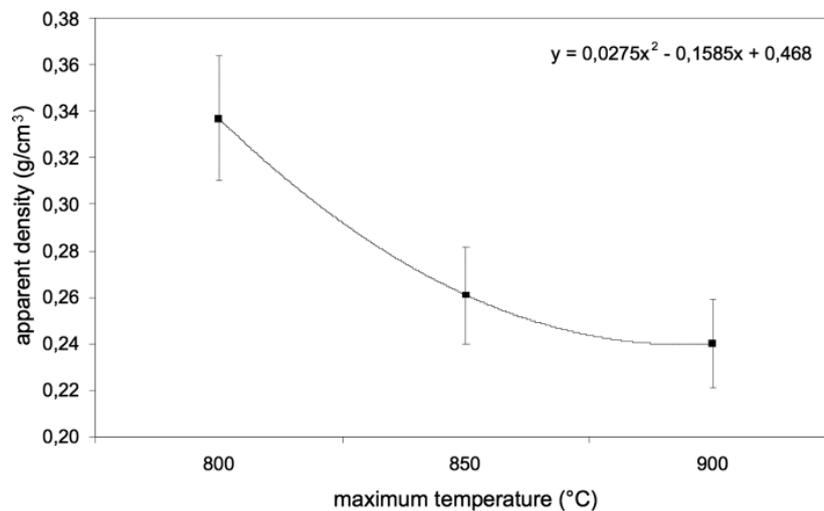
Figure 1. Evolution of the apparent density of the ceramic foam due the firing temperature
