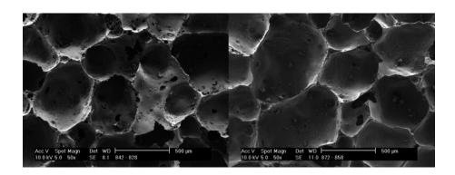
Figure 2. Microstructure after sintering for 850°C and 900°C firing temperatures
