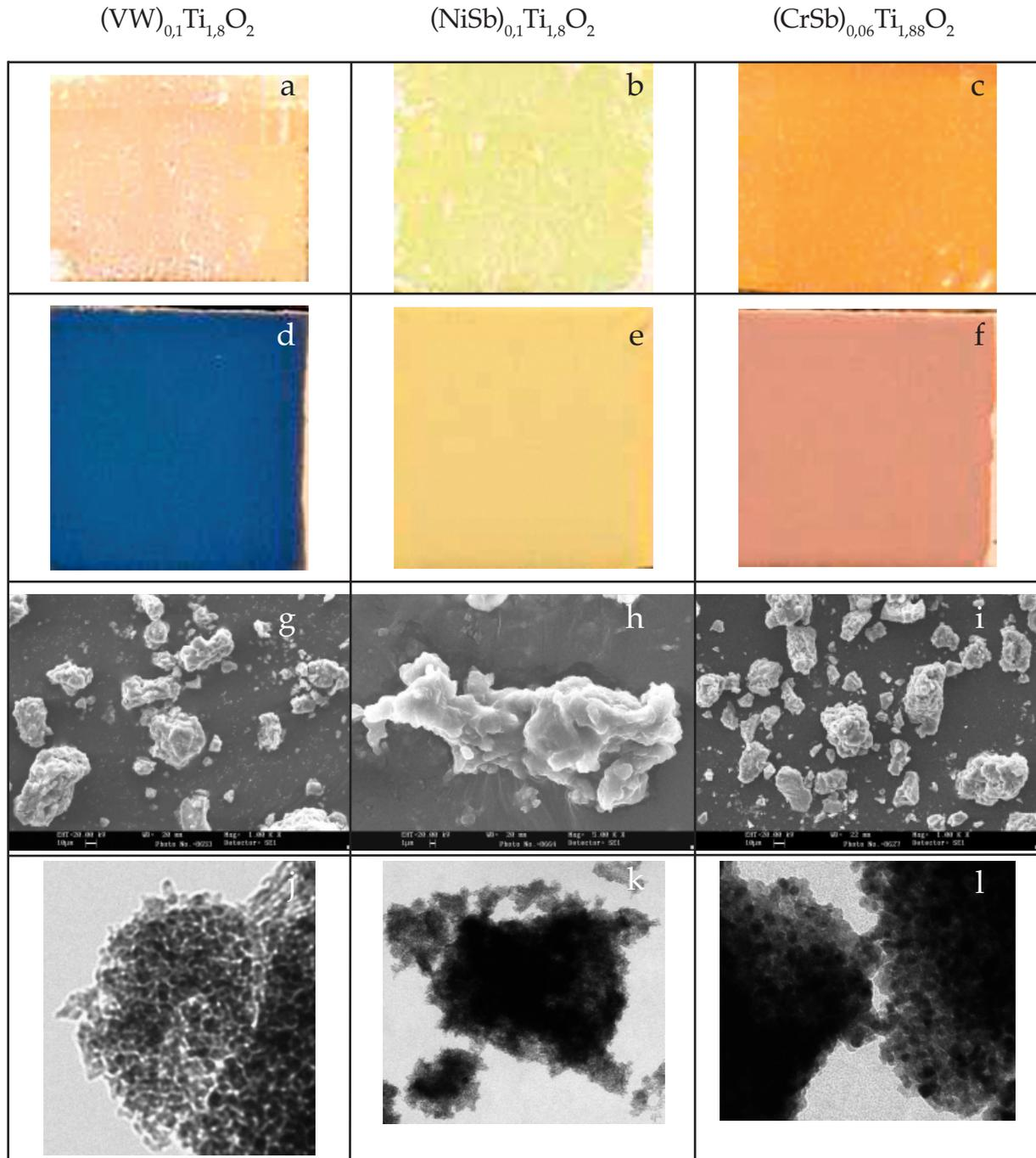
Figure 1. (a, b, and c) Photograph of the screen printed powders on porcelain tile body, (d,e,f) Photograph of the glazed samples in conventional porous single-fired wall tile frit powders fired at the indicated temperature, (g,h,i) SEM micrographs of the dry green (j,k,l). TEM micrographs of samples stabilised at 500°C (j and l) or dry samples (k).
