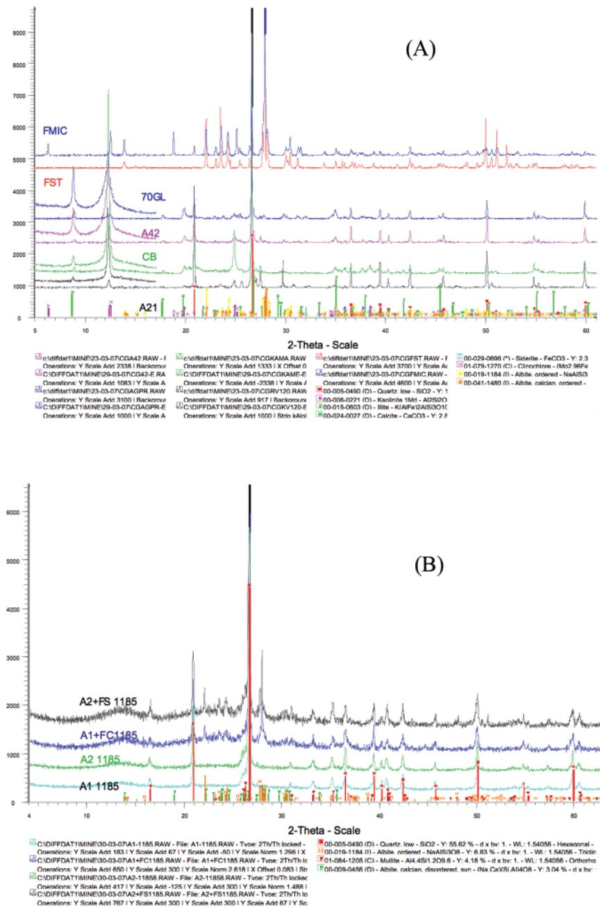
Figure 1. Diffractogram of raw materials (A) and diffractogram of fired bodies (B).
