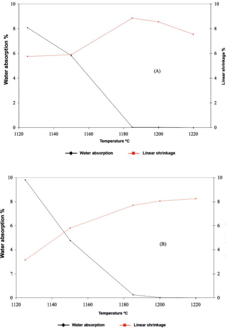
Figure 2. Vitrification diagram of body A1+FC (A) and of body A2+FS (B).
