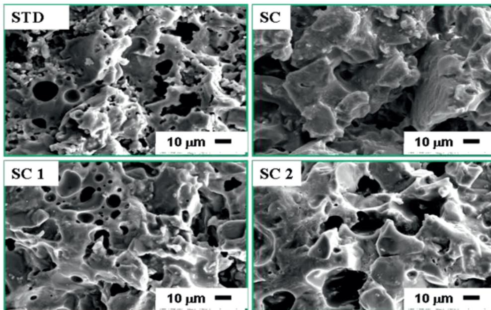
Figure 3. Representative SE images of the fractured and etched surfaces of the investigated formulations (cycle: 1150°C, 32 min.).
