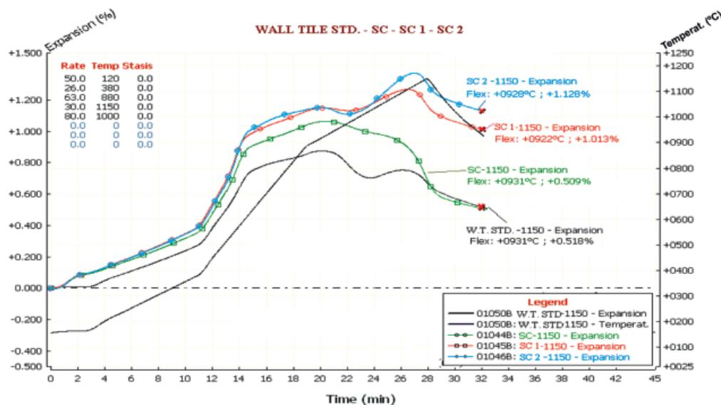
Figure 1. Dilatometric curves of the standard wall tile and investigated formulations (cycle: 1150°C, 32 min.).
