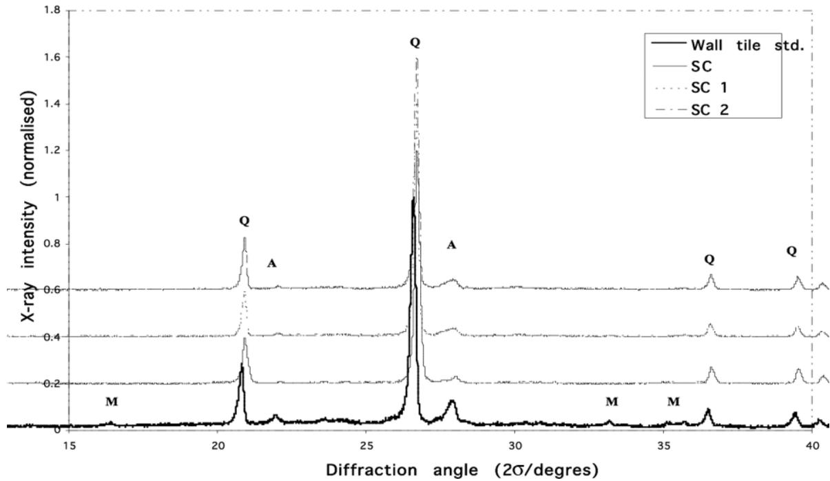
Figure 2. XRD spectra of the investigated fired bodies (cycle: 1150°C, 32 min.)
