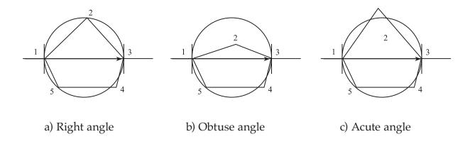
*Figure 6. Graphic examples that illustrate the determination of the type of angle for vertex 2: a) for a right angle; b) for an obtuse angle and c) for an acute angle.*
