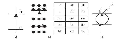
*Figure 4. a) Fine RS for qualitative orientation; b) the iconic representation in which each symbol corresponds is as follows: l: left, r: right, f: front, s: straight, m: middle b: back, i: identical; c) fine RS for orientation augmented by a circle with diameter ab.*
