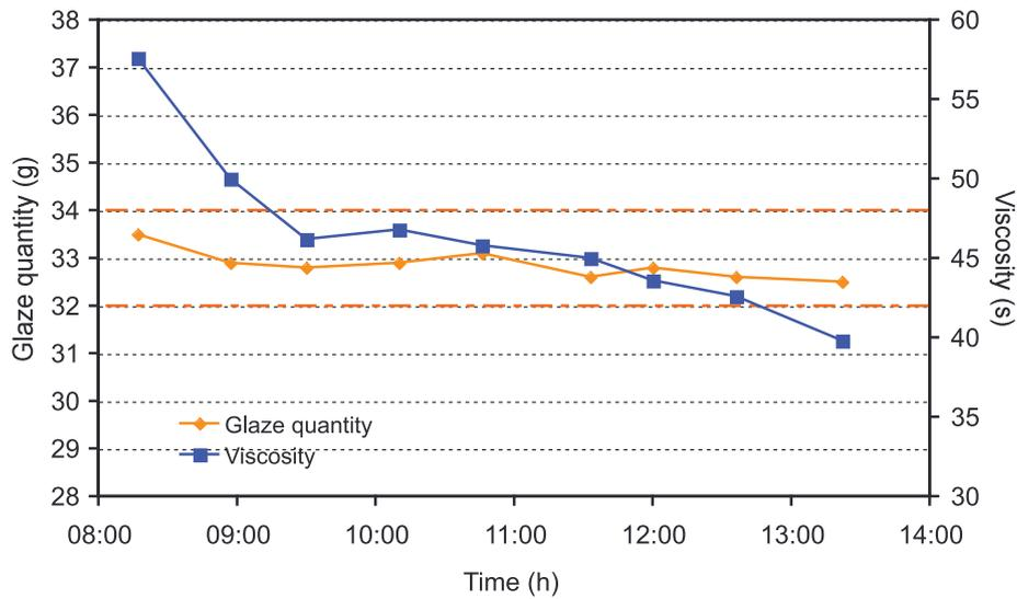
Figure 9. Evolution with time of applied glaze viscosity and quantity using the feed system developed in this study, under industrial conditions.
