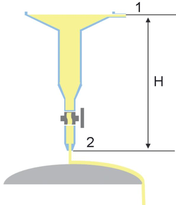
Figure 1. Scheme of a generic glaze feed system to which a mechanical energy balance is applied between points 1 and 2.
