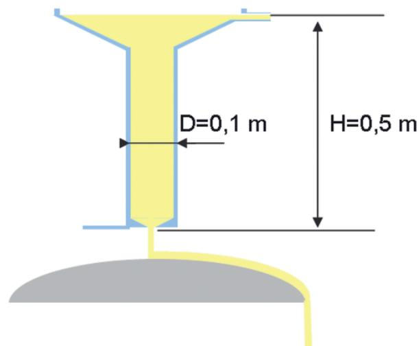
Figure 2. Scheme of the developed feeder prototype.
