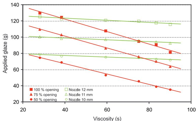
Figure 4. Evolution of the glaze quantity applied on to 33x33 cm tiles as a function of glaze viscosity for the developed prototype (green line and empty points) and for a conventional glaze feed system (red line and solid points).
