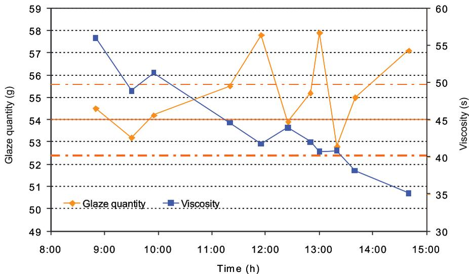
Figure 8. Evolution with time of applied glaze viscosity and quantity using a conventional feed system, under industrial conditions.
