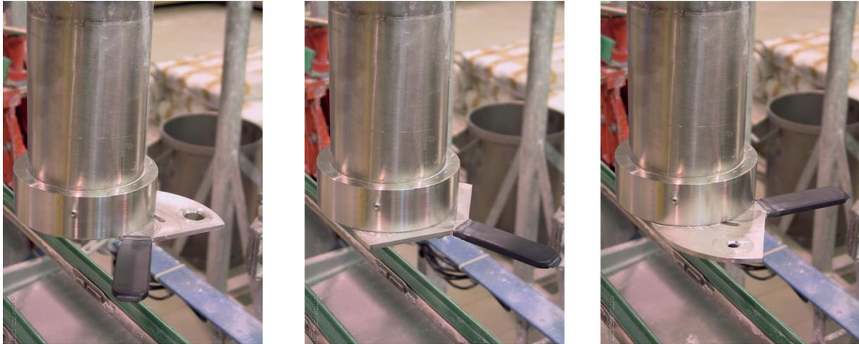
Figure 3. Detail of the rapid nozzle changeover system in its three positions: (from left to right) nozzle 1, closed, and nozzle 2.
