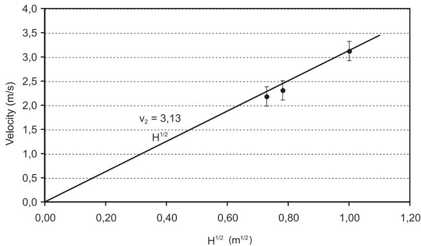
Figure 6. Dependence between glaze discharge rate and glaze height. Fit of the experimental results to Equation 5.
