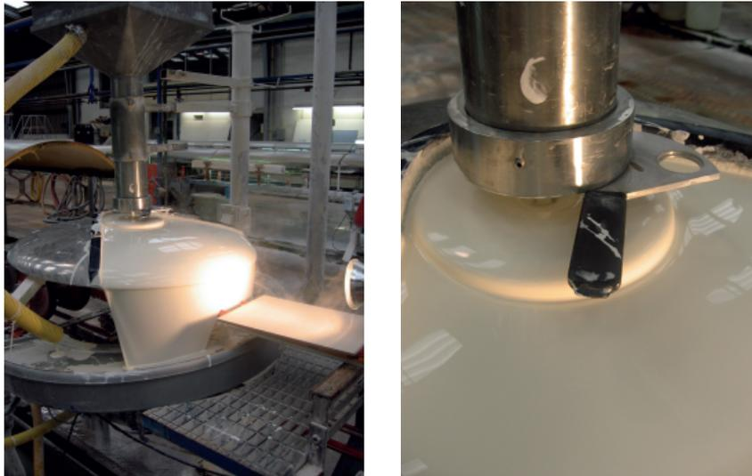
Figure 7. Prototype installed in the industrial glazing line (left) and detail of the rapid nozzle changeover system (right).
