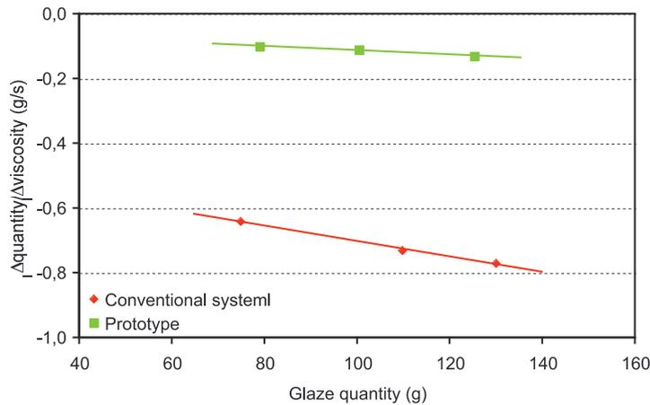
Figure 5. Variation of sensitivity to the changes in viscosity of the feeders studied with the applied quantity of glaze.
