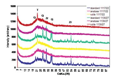
Figure 4. XRD patterns for 5% TiO<sub>2</sub> addition (anatase and rutile glazes) at  $1117^{\circ}$ C/22min and  $1130^{\circ}$ C/27min firing cycles (Q=quartz; T=titanite; Zr=zircon)
