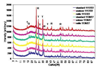
Figure 6. XRD patterns for 15%  $TiO_2$  addition (anatase and rutile glazes) at  $1117^{\circ}$ C/22min and  $1130^{\circ}$ C/27min firing cycles (A=anatase; Q=quartz; T=titanite; Zr=zircon)
