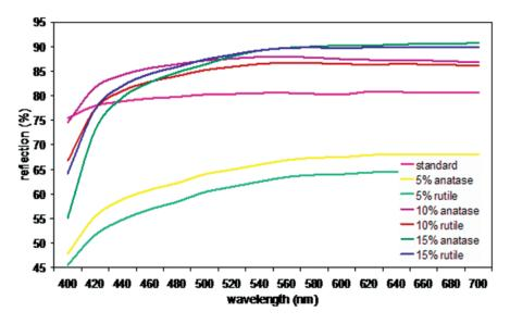
Figure 3. Reflectance spectra for 5%, 10% and 15% anatase and rutile glazes fired at 1130°C/27min cycle
