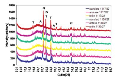
Figure 5. XRD patterns for 10% TiO<sub>2</sub> addition (anatase and rutile glazes) at  $1117^{\circ}$ C/22min and  $1130^{\circ}$ C/27min firing cycles (A=anatase; Q=quartz; T=titanite; Zr=zircon)
