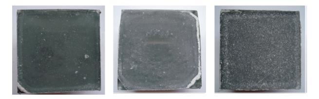
*Figure 4. (a) Interfacial mode of rupture for control glass tile and (b) for vinylsilane modified surface. (c) Mixed mode interfacial-cohesive failure of the mortar due aminosilane glass tile modification.*
