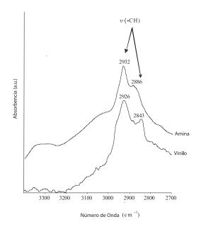
Figure 2. FTIR spectra for the modified glass surface.
