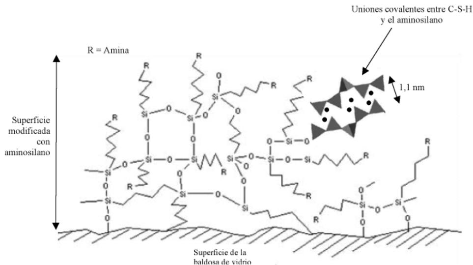
Figure 5. Possible interactions between aminosilanes and Portland cement.
