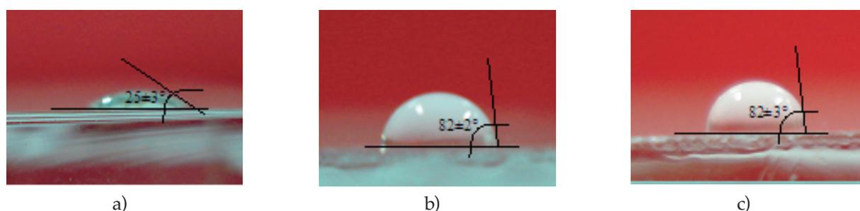
Figure 1. Contact angle measurements for control (unmodified) (a), amine (b), and vinyl (c) silane modified glass tiles.
