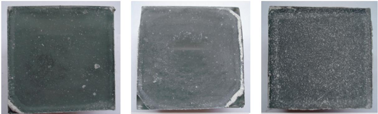
Figure 4. (a) Interfacial mode of rupture for control glass tile and (b) for vinylsilane modified surface. (c) Mixed mode interfacial-cohesive failure of the mortar due aminosilane glass tile modification.
