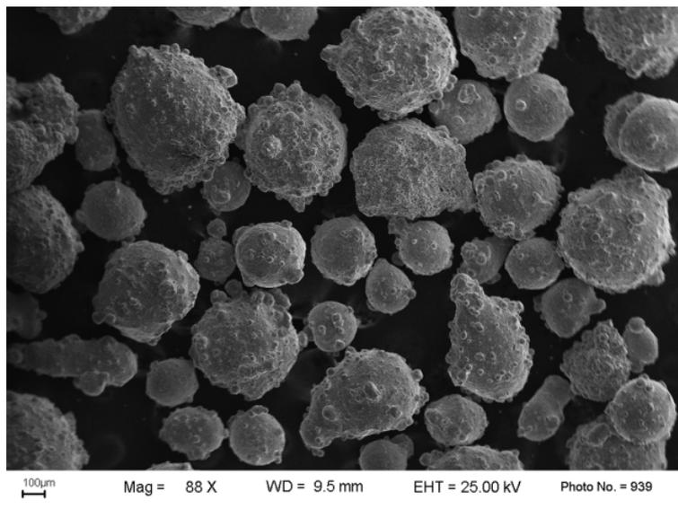
Figure 1. SEM micrograph of the stainless-steel particles.
