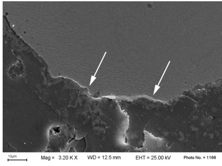
Figure 5. SEM micrographs of the polished surface of Mix 3, crack path blunted by a metal particle. The arrows underline the metal detachments.
