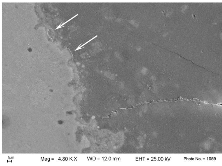
Figure 4. SEM micrographs of the polished surface of Mix 2, crack path blunted by a metal particle. The arrows underline the metal detachments.
