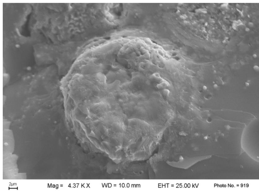
Figure 2. SEM micrograph of Mix 2, a round metal particle adhering well to the ceramic matrix.
