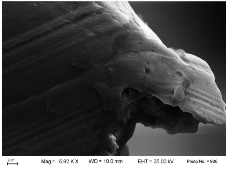
Figure 3. SEM micrograph of Mix 3, showing the elongated deformed area of the metal particle.
