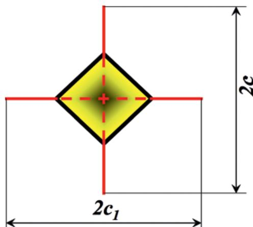
Figure 3. Vickers impression and median-radial cracks.
